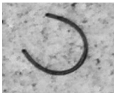
Figure 22 CP sausage bent to a horse shoe shape on x-ray film, width = 0.19 mm [16]
