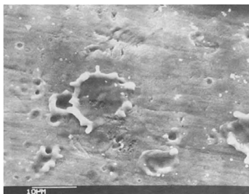
Figure 5 Impact marks of small CPs hitting a titanium target [2]
