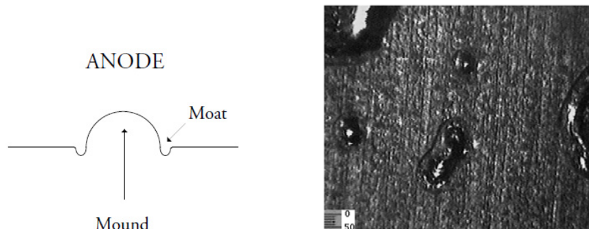
Figure 41 Deposits and ionization moat left by CP impacts on the anode; Left: Cross section; Right: photo
