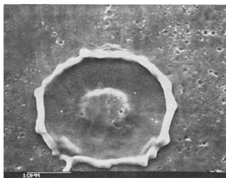
Figure 16 Ring mark of a CP with wiping [2]
