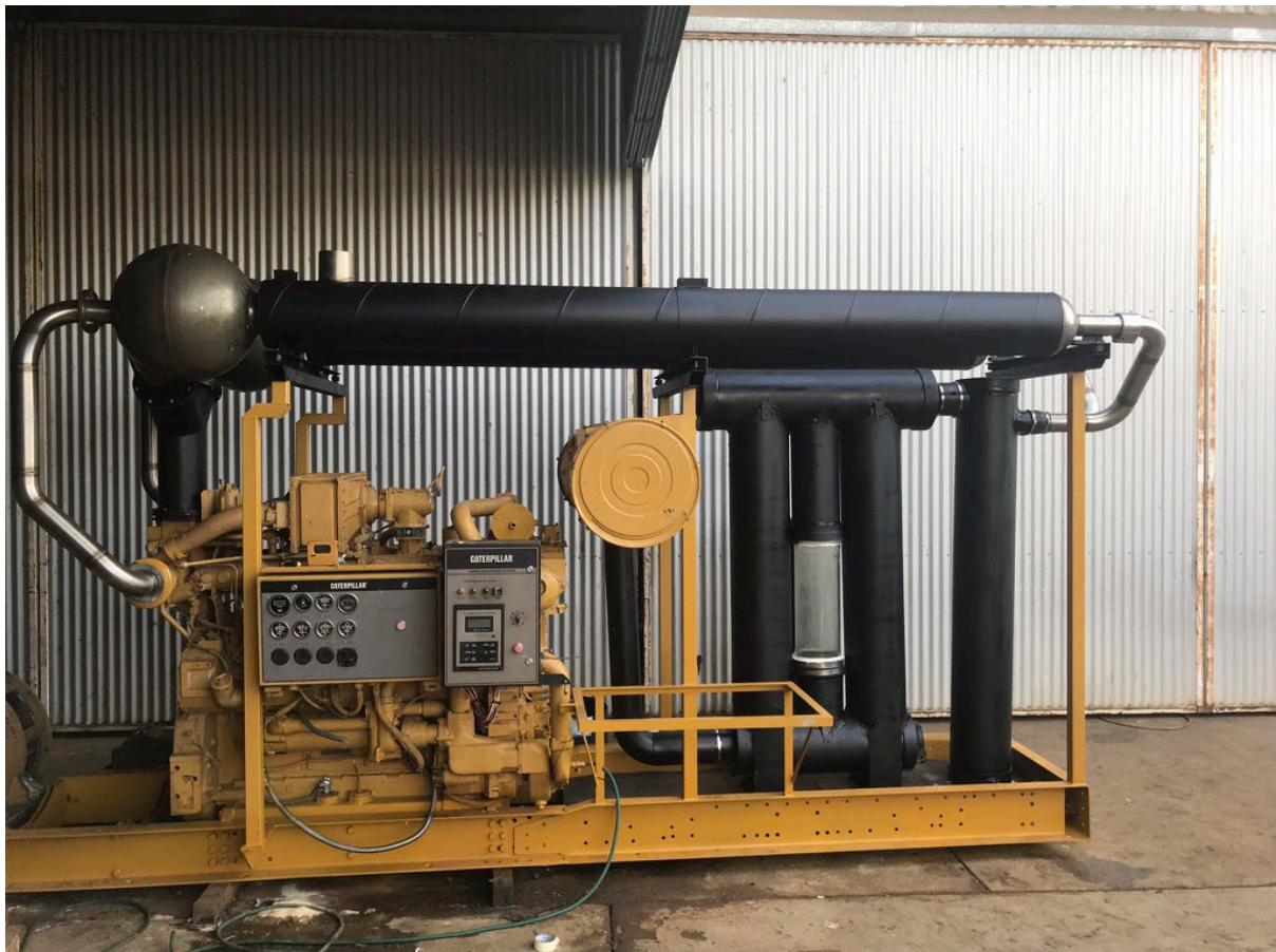
DIAGRAM 65 - BELOW - PHOTO OF OUR CATERPILLAR G3508 E 670 Hp V8 GAS 8:1 COMPRESSION RATIO ENGINE WITH THE THUNDERSTORM GENERATOR TECHNOLOGY FITTED GENERATING MORE POWER AND ZERO CARBON MONOXIDE AND WASTE HYDROCARBONS IN THE EXHAUST STREAM. IN ADDITION THE EXHAUST GAS TEMPERATURE MAY BE REDUCED BY UP TO 20 TIMES DOWN TO AMBIENT LEVELS.
