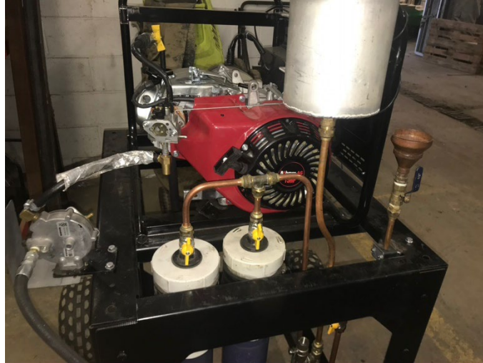
DIAGRAM 35 - THE THUNDERSTORM GENERATOR TEST SET UP FROM LEFT TO RIGHT IS THE GAS REGULATOR SUPPLYING PROPANE, THEN THE TWO MSAART EVO GENERATORS WITH THE WHITE CAPS AND YELLOW VALVES THEN ABOVE IS THE IONIZER PROVIDING UV TREATED ATMOSPHERIC AIR THEN THE FILLER FUNNEL FOR THE LEACHATE. THE 380CC SINGLE CYLINDER 4 STROKE ENGINE IS IN THE BACKGROUND. PAGE 1 SHOWS THE FRONT VIEW OF THE ENGINE.
