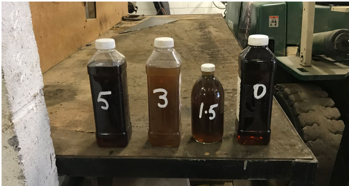
DIAGRAM 32 - THE BOTTLES FROM LEFT TO RIGHT ARE THE 5 MINUTE, 3 MINUTE, 1.5 MINUTE AND A ZERO MINUTE CONTROL SAMPLE. THE 3 MINUTE SAMPLE IS LIGHTER THAN THE CONTROL.
