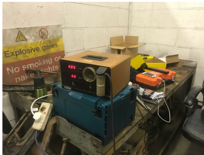
DIAGRAM 36 - THE BOSCH EXHAUST GAS ANALYSER MEASURING ZERO EMISSIONS OF CARBON MONOXIDE AND HYDROCARBONS AFTER TREATMENT OF THE EXHAUST FUMES WITHIN THE CATALYTIC TORNADO RESONATOR (CTR) ASSEMBLY OF AIR PULLED THRU BY THE VACCUM MADE BY THE ENGINE. WHEN THE ENGINE IS JUST RUN NORMALLY ON GAS THE CARBON MONOXIDE LEVELS ARE ABOUT 2% AND THE HYDROCARBON LEVEL IS BETWEEN 1,000 TO 3,000 PPM DEPENDING ON THROTTEL SETTINGS.
